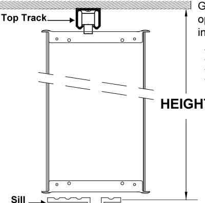
Gates are manufactured to fit the cab opening. Precise measurements will insure a proper fit.
