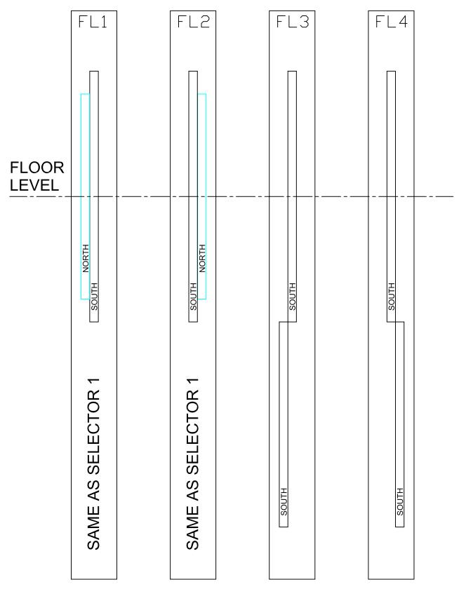
After magnets are positioned, trim as necessary to avoid a "yo-yo" effect during arrival to a floor.
